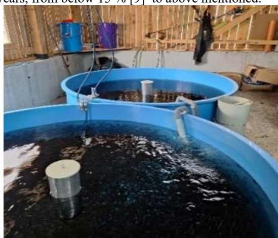
Figure 10. Use of pure oxygen for rearing trout fry, injected into the water via ceramic micro-bubble diffusers – Tropic Ribarstvo, Bosnia and Herzegovina, Republika Srpska (Photo: N. Savić, 2024)
