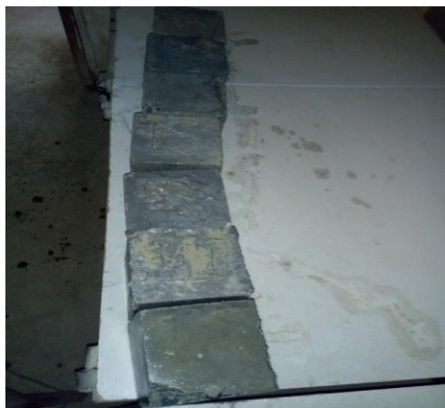
Plate 4. Blended concretes at different replacement levels after curing ready for crushing
