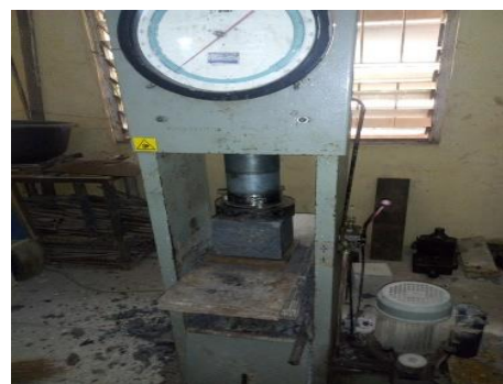
Plate 6. Crushing the concrete for compressive strength measurement
