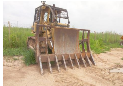
Fig. 6. Crawler tractor mounted with raking Blade for land developmet windrowing, raking and root de-stumping
