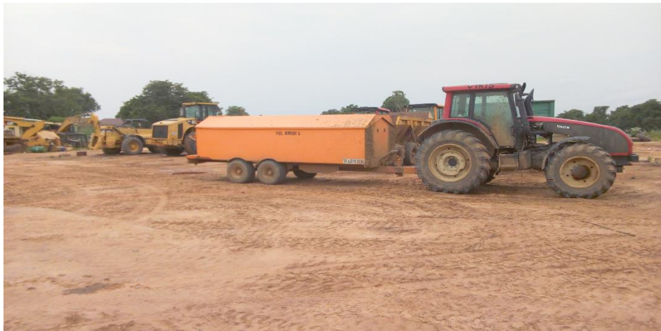
Fig.13. A fuel bowser for supplying fuel from one pump station to another
