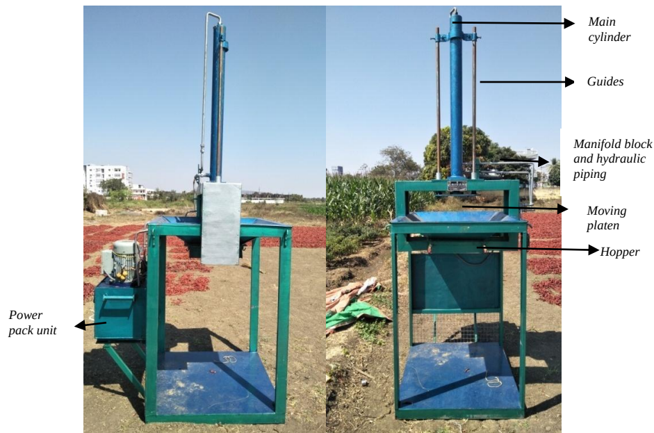
Figure 2. Mechanical dried chillies compaction and bagging machine
