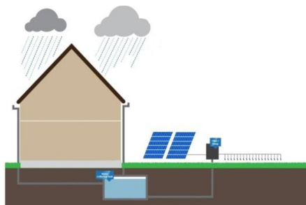
Figure 1. Combining the rainwater harvesting with solar irrigation
