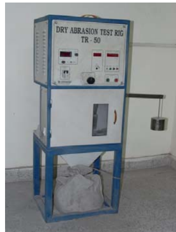
Figure 1. Rubber wheel /dry sand abrasion test apparatus
