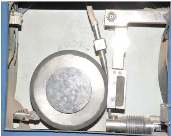
Figure 1. Rubber wheel /dry sand abrasion test apparatus
