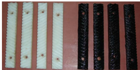
Figure 2. Comparison of nylon and cast iron rasp bars
