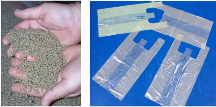
Figure 2. Granulated material and new, regenerated films
