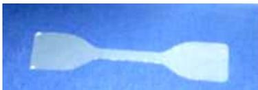
Figure 3. A sample for the tensile test
