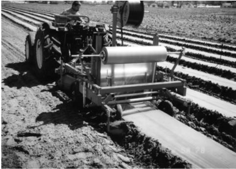
Figure 1: Ridge forming and foil laying machine type AF1
