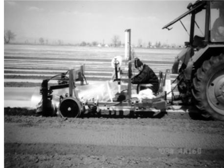
Figure 2: Tunnel-foil laying machine type AFF-1000
