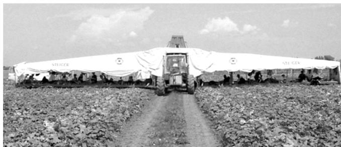
**Figure 3:** Belt cucumber picking carriage type STEIGER
