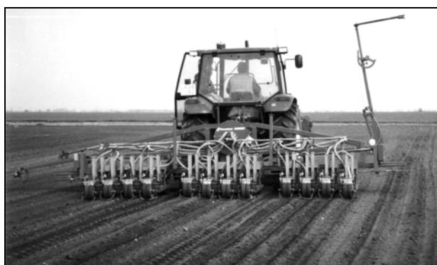
Figure 1: ACCORD MINIAIR SUPER pneumatic direct seeder
