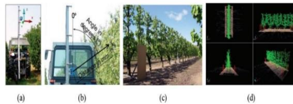
Figure 9. The LIDAR measurement system, (a) data in Cartesian coordinates, (b) data in polar coordinates (c) pear orchard, (d) different views of the 3D structure.
