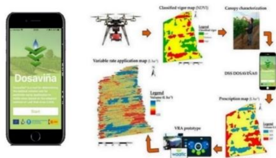
Figure 3. Left: image of DOSAVINA DSS, free available APP (Android and ISO) to determine the optimal application rate for vineyard plantations; right: cycle of VRA based on canopy imagery generated with UAV. The system has been proven to reduce PPP from 15 to 40% depending on the conditions.
