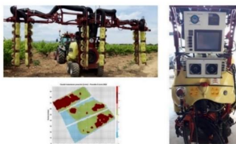
Figure 5. VRA sprayer developed within PIVOS project. The system is equipped with PWM nozzles to follow the prescription map previously developed after satellite imagery.
