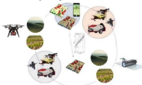
Figure 4. VRA cycle developed within PIVOS project, UAV and satellites have been used to generate accurate correlation to estimate canopy parameters. Furthermore, based on values these values, VRA technologies have been already implemented in field conditions, IN all case it has been demonstrated a promising technology with good results in terms of PPP reduction.
