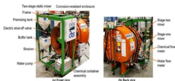
Figure 12. Attachment of components of the premixing in-line injection system to the laser-guided variable-rate orchard sprayer.
