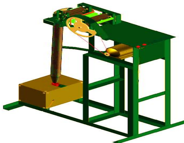
Fig. 4. Integrated broom peeling-tethering processing machine, [8].
