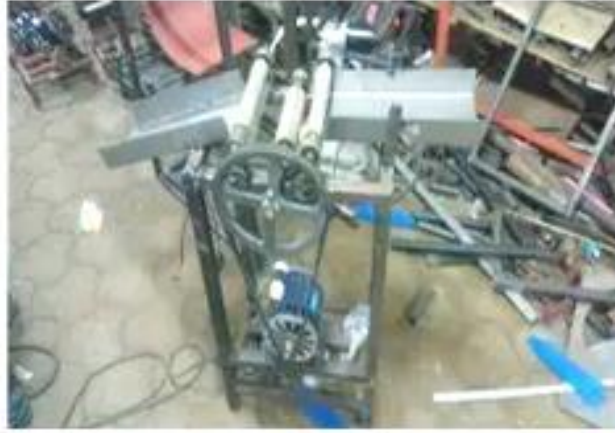
Fig. 3. Novel machine to separate midribs from coconut leaflets, [7].
