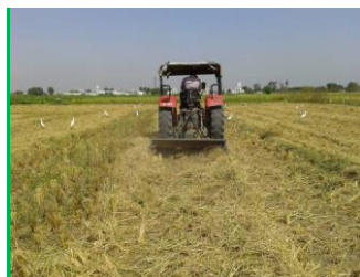
Figure 1. A view of stubble shaver machine
