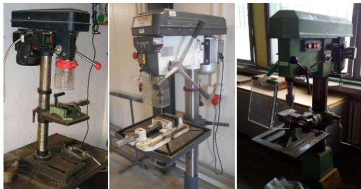
Slika 1. Bušilice opremljene zaštitnikom oko reznog alata (sopstveni izvor) Figure 1. Drilling machine equipped with safety guard around the cutting tools (Authors source)
