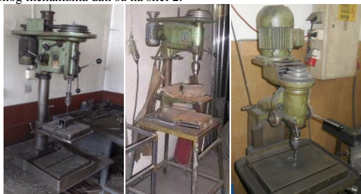
Slika 2. Bušilice koje nisu opremljene zaštitnikom oko prenosnog mehanizma (sopstveni izvor) Figure 2. Drilling machines not equipped with a safety gear around the transmission (Authors source)
