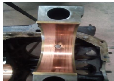
Slika 38. Pogled na neoštećeni ležaj kolenastog vratila 11682/17445 Figure 38. View of undamaged crankshaft bearing
