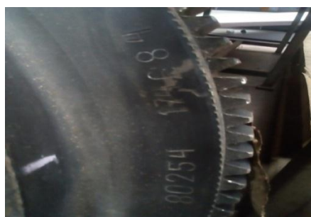
Slika 7. Zamajac 80254/174684 - oznaku zamajca i oštećenja zubaca Figure 7. Flywheel 80254 /174684 - a flywheel marking and tooth damage
