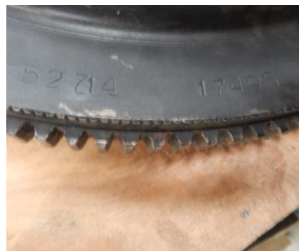
Slika 22. Zamajac 52714/17495 -pogled na oznaku zamajca i na oštećene zupce zamajca Figure 22. Flywhel 52714/17495 - view of the mark and tooth damage
