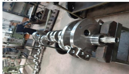
Slika 6. Kolenasto vratilo 90325/76700 bez pokretnih masa Figure 6. Crankshaft 90325/76700 -view of a complete crankshaft without moving masses
