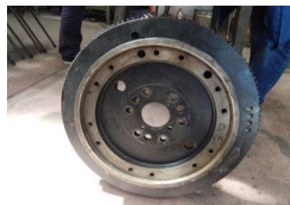
Slika 12. Zamajac 23645/17817 -pogled sa strane kojom se spaja sa kolenastim vratilom Figure 12. Flywheel 23645/17817 -view of the flywheel from the side that connects to the crankshaft
