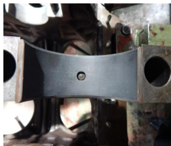
Slika 30. Pogled na neoštećen ležaj kolenastog vratila 90325/76700 Figure 30. View of undamaged crankshaft bearing 90325/76700
