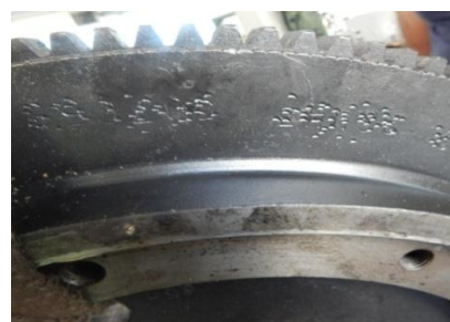
Slika 14. Zamajac 23645/17817 -pogled na oznaku zamajca Figure 14. Flywheel 23645/17817 - view of flywheel marking and tooth damage
