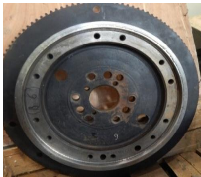
Slika 21. Zamajac 52714/17495 -pogled na oznaku zamajca i na oštećene zupce zamajca Figure 21 Flywhel 52714/17495 - view of the mark and tooth damage
