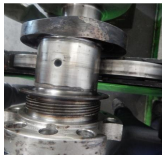
Slika 24. Kolenasto vratilo 90325/76700 -pogled na zapušenom otvoru dovoda maziva prvog rukavca kolenastog vratila Figure 24. Crankshaft 90325/76700 - view of the clogged lubricant supply port of the first crankshaft sleeve
