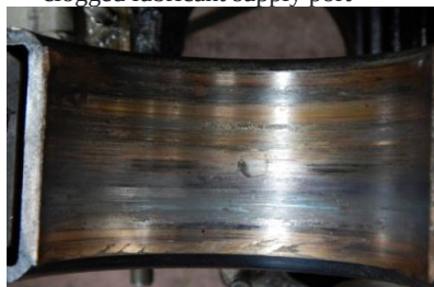
Slika 37. Kolenasto vratilo 11682/17445 -pogled na zapušenom otvoru dovoda maziva prvog rukavca kolenastog vratila Figure 37. Crankshaft 11682/17445 - view of the clogged lubricant supply opening of the first crankshaft arm
