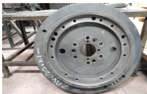
Slika 8. Zamajac 23645/17817 -strana koja se spaja sa kolenastim vratilom Figure 8. Flywheel 23645/17817 -view of the flywheel from the side that connects to the crankshaft
