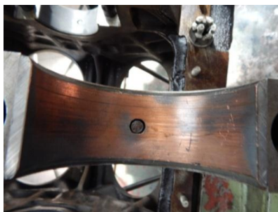
Slika 29. Pogled na oštećen ležaj kolenastog vratila 90325/76700 Figure 29. View of damaged crankshaft bearing 90325/76700
