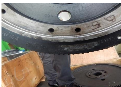
Slika 13. Zamajac 23645/17817 -pogled na broj zamajca Figure 13. Flywheel 23645/17817 -view of flywheel marking and tooth damage
