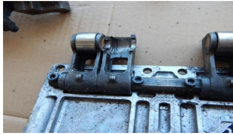
Slika 13. Oštećeno ležište rolnice koja usmerava kredanje šipke podizača šestog izduvnog ventila motora Figure 13. A damaged roll bearing that directs the choke of the sixth exhaust valve of the engine
