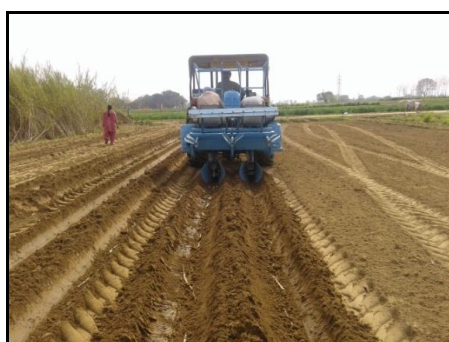
Figure 5. View of sugarcane cutter planter with set covering unit raised
