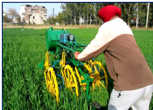
Figure 3. Real and field operational view of self propelled spoke wheel nitrogen applicator
