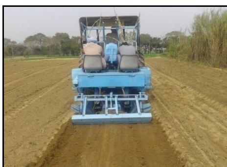
Figure 6. View of sugarcane cutter planter with covering unit lowered
