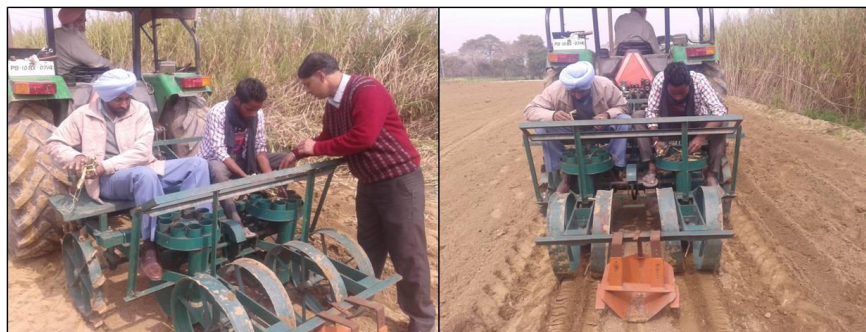
Figure 3. View of Napier-Bajra sowing with two row semi-automatic vegetable nursery transplanter
