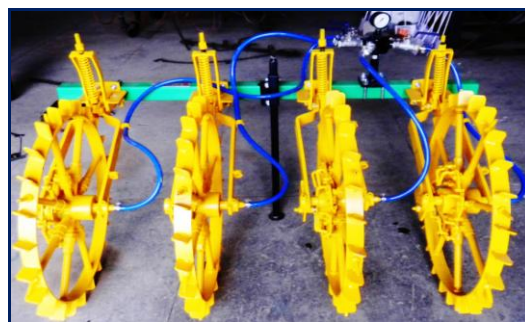
Figure 2. View of self propelled spoke wheel nitrogen applicator
