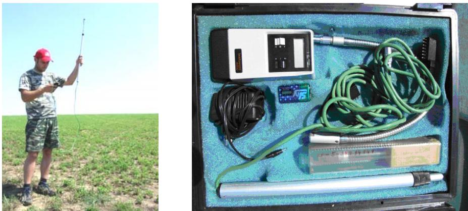
Figure 3. Anemometer Testovent 4000
