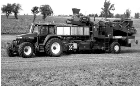
*Fig. 1. Harvester Grimme SE 150 -60 with a device for filling and transferring the box (developed by Schoepstal Maschinenbau GmbH [7])*
