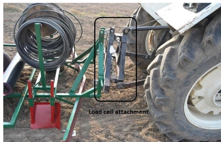
Fig. 10. Measuring draft using Monard Digitalizer load cell
