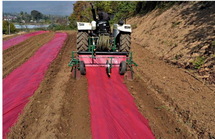
Fig. 9. An overview of operation of tractor operated mulch laying machine
