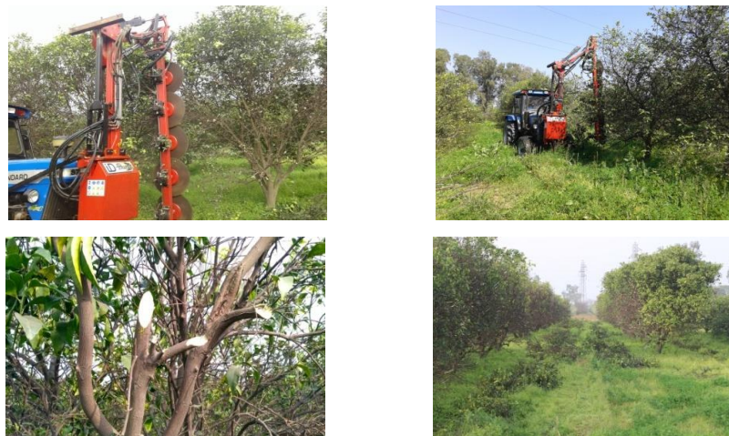
Fig. 10. Sequential view of Tractor operated Pre pruner in vertical cutting position and view of cut branches
