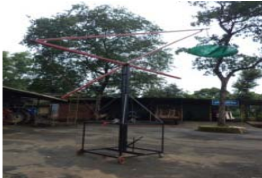
Figure 2. Assembled view of developed tree shaker
