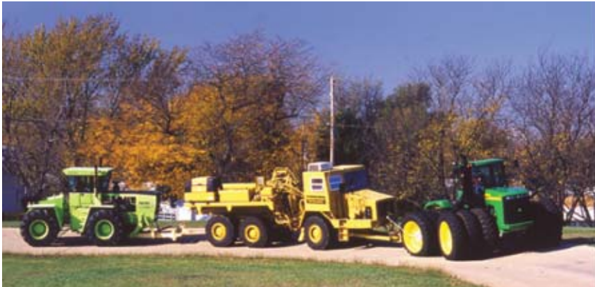
Figure 2. The lead tractor is being tested on the track during drawbar performance tests The two vehicles in tow are load units.
