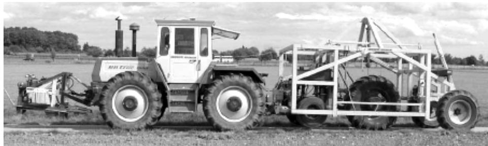
Figure 4: The single wheel tester.
