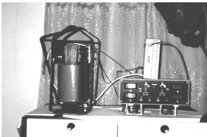
Sl. 3. Elektromagnet MOV-2 i kontrolni instrument KU-1-MOV
